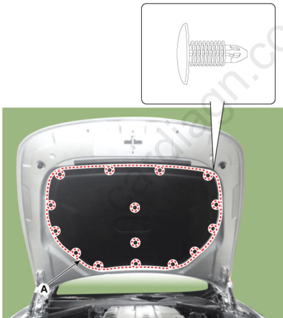
2. Remove the hood garnish (A) after loosening the mounting nuts.
